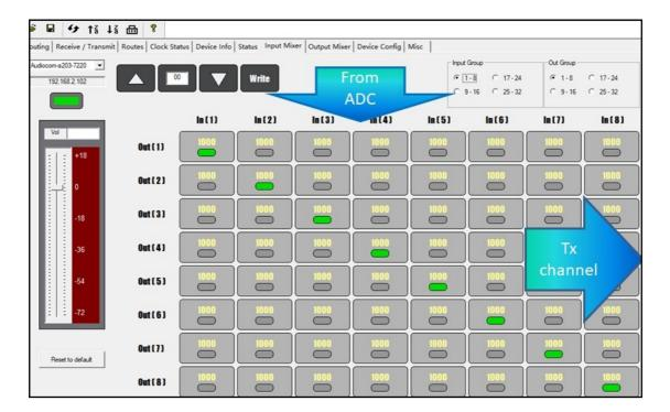
The vertical representation in the diagram shows each audio channel fed into the module by the ADC (or DSP) and ready to be transmitted over the network. The input audio is arranged from left to right, and the number of channels represented is also determined by the input group selector. Routes 1-8 are shown in the figure.
