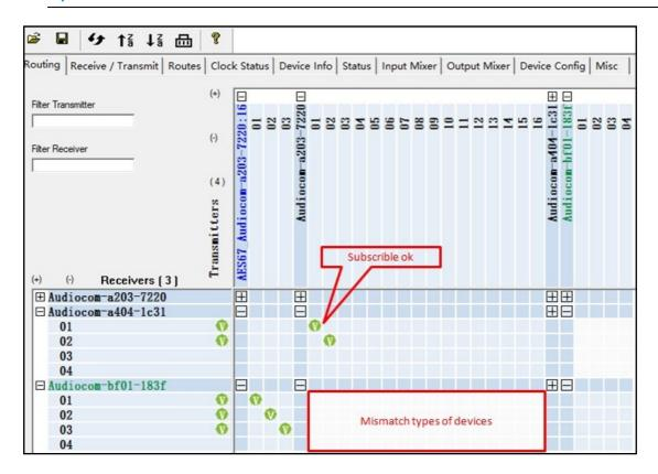
If the grid for some channel intersections is gray-white and clicking does not work, the channel between the two modules is not subscribeable. There are several reasons for this:
