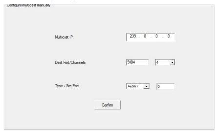
Normally, multicast does not require a source port to be set. For some special types of multicast, such as multicast transmitted by Dolby devices, it uses the source port to distinguish different multicasts, and the source port needs to be added here. For multicast with a source port set, AudioGridController starts with Dolby when displaying the name and identifies it with the source port at the end to distinguish it from other multicasts.
